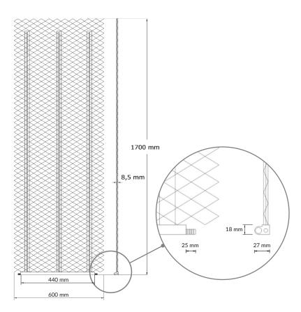
The hybrid surface heating system concealed under plaster (1,5 cm) has been designed on the basis of many years of research on the use of the active radiator technology in heating applications. 3THERMO eliminates all the current disadvantages of wall heating solutions:
